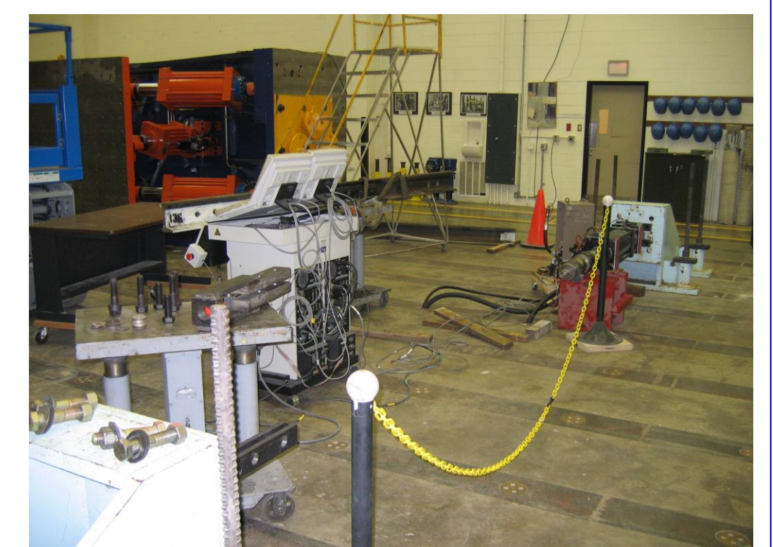
Test area, showing reaction blocks and actuator
